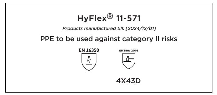
is in conformity with the provisions of Regulation (EU) 2016/425 and with the standards EN 16350:2014, EN 388:2016 +A1:2018, EN ISO 21420:2020 and is identical to the PPE which is subject to the EU-Type examination (Module B, Annex V of the Regulation), under certificate number 032/2022/0791, issued by the Notified Body:
