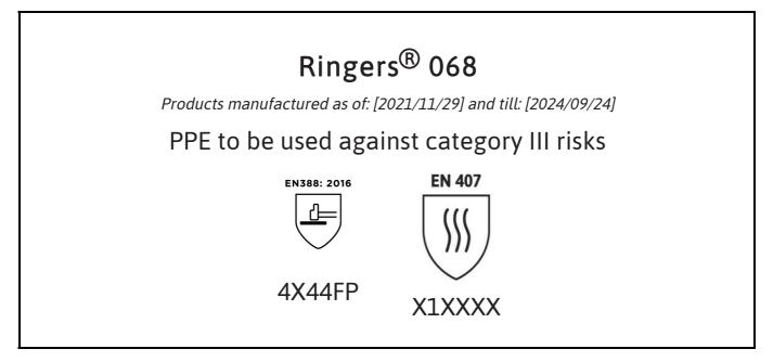
is in conformity with the provisions of Regulation (EU) 2016/425 and with the standards EN 388:2016 +A1:2018, EN407:2020, EN ISO 21420:2020 and is identical to the PPE which is subject to the EU-Type examination (Module B, Annex V of the Regulation), under certificate number 032/2021/1269, issued by the Notified Body:
