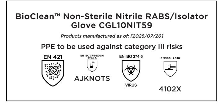
is in conformity with the provisions of Regulation 2016/425 on personal protective equipment, as amended to apply in GB, and with the standards EN 421:2010, EN ISO 374-1:2016, EN ISO 374-5:2016, EN 388:2016 +A1:2018 and is identical to the PPE which is subject to the Type-examination (Module B, Annex V of the Regulation), under certificate number 032/2024/0182, issued by the Body:
