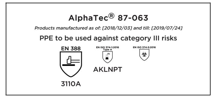
is in conformity with the provisions of Regulation (EU) 2016/425 and with the standards EN 388:2016, EN 420:2003 + A1:2009, EN ISO 374-1:2016, EN ISO 374-5:2016 and is identical to the PPE which is subject to the EU-Type examination (Module B, Annex V of the Regulation), under certificate number 032/2018/1930, issued by the Notified Body:
