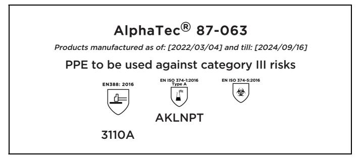
is in conformity with the provisions of Regulation (EU) 2016/425 and with the standards EN 388:2016 +A1:2018, EN ISO 21420:2020, EN ISO 374-1:2016, EN ISO 374-5:2016 and is identical to the PPE which is subject to the EU-Type examination (Module B, Annex V of the Regulation), under certificate number 032/2022/0330, issued by the Notified Body:
