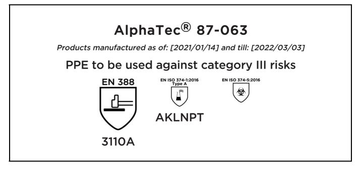
is in conformity with the provisions of Regulation (EU) 2016/425 and with the standards EN 388:2016, EN 420:2003 + A1:2009, EN ISO 374-1:2016, EN ISO 374-5:2016 and is identical to the PPE which is subject to the EU-Type examination (Module B, Annex V of the Regulation), under certificate number 032/2018/1930.02, issued by the Notified Body:
