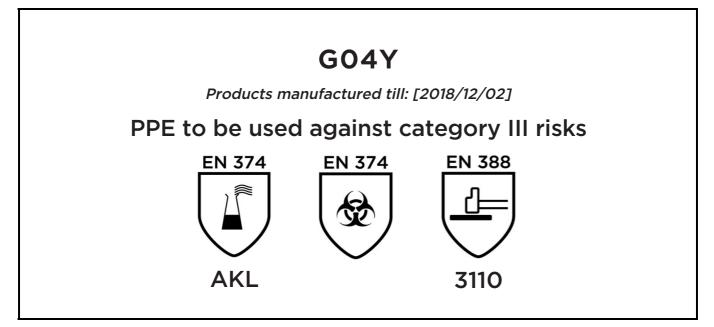
is in conformity with the provisions of Regulation (EU) 2016/425 and with the standards EN 374:2003, , EN 388:2003, EN 420:2003 + A1:2009 and is identical to the PPE which is subject to the EC Type examination; under certificate number CE 602716 issued by the Notified Body:
