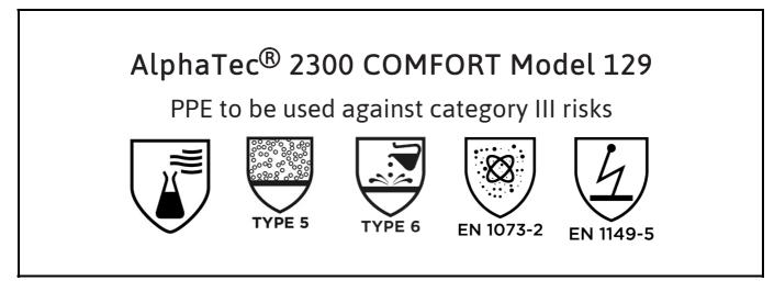
is in conformity with the provisions of Regulation (EU) 2016/425 and with the standards, EN ISO 13982-1:2004 + A1:2010, EN 13034:2005 + A1:2009, EN 1073-2:2002, EN 1149-5:2018, EN ISO 13688:2013 (with exception of puncture resistance for which class 1 was achieved) and is identical to the PPE which is subject to the EU-Type examination (Module B, Annex V of the Regulation), under certificate number 0598/PPE/24/4483, issued by the Notified Body:
