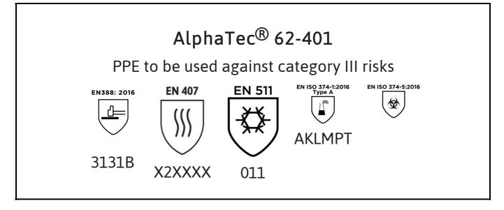
is in conformity with the provisions of Regulation 2016/425 on personal protective equipment, as amended to apply in GB, and with the standards EN 388:2016 +A1:2018, EN407:2020, EN 511:2006, EN ISO 21420:2020, EN ISO 374-1:2016, EN ISO 374-5:2016 and is identical to the PPE which is subject to the UK Type-examination (Module B, Annex V of the Regulation), under certificate number AB0321/25478-01/E00-00, issued by the Approved Body:
