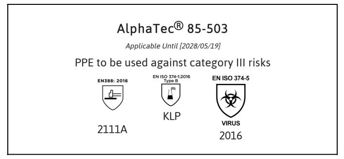
is in conformity with the provisions of Regulation 2016/425 on personal protective equipment, as amended to apply in GB, and with the standards EN 388:2016 +A1:2018, EN ISO 21420:2020, EN ISO 374-1:2016, EN ISO 374-5:2016 and is identical to the PPE which is subject to the UK Type-examination (Module B, Annex V of the Regulation), under certificate number AB0321/24204-01/E00-00, issued by the Approved Body:
