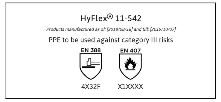
is in conformity with the provisions of Regulation (EU) 2016/425 and with the standards EN 388:2016, EN 407:2004, EN 420:2003 + A1:2009 and is identical to the PPE which is subject to the EU-Type examination (Module B, Annex V of the Regulation), under certificate number 032/2018/1414, issued by the Notified Body:
