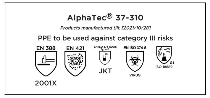
is in conformity with the provisions of Regulation (EU) 2016/425 and with the standards EN 388:2016, EN 420:2003 + A1:2009, EN 421:2010, EN ISO 374-1:2016 Type B, EN ISO 374-5:2016, ISO 18889:2019 and is identical to the PPE which is subject to the EU-Type examination (Module B, Annex V of the Regulation), under certificate number 032/2019/1520.02, issued by the Notified Body:
