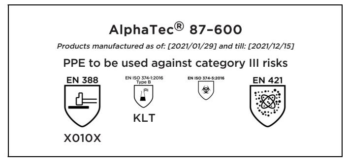
is in conformity with the provisions of Regulation (EU) 2016/425 and with the standards EN 388:2016, EN 420:2003 + A1:2009, EN ISO 374-1:2016 Type B, EN ISO 374-5:2016, EN 421:2010 and is identical to the PPE which is subject to the EU-Type examination (Module B, Annex V of the Regulation), under certificate number 032/2018/1713.02, issued by the Notified Body:
