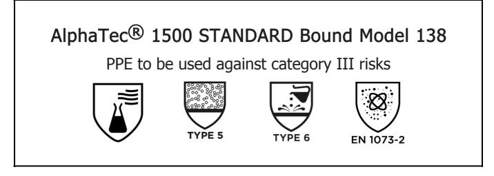
is in conformity with the provisions of Regulation (EU) 2016/425 and with the standards EN ISO 13688:2013, , EN ISO 13982-1:2004 + A1:2010, EN 13034:2005 + A1:2009, EN 1073-2:2002 (with exceptions for puncture resistance being class 1 and resistance to ignition not tested) and is identical to the PPE which is subject to the EU-Type examination (Module B, Annex V of the Regulation), under certificate number 0598/PPE/24/2247, issued by the Notified Body:
