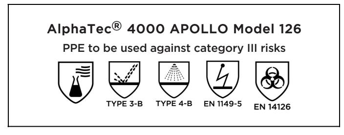
is in conformity with the provisions of Regulation (EU) 2016/425 and with the standards, EN 14605:2005 + A1:2009, EN 1149-5:2018, EN 14126:2003, EN ISO 13688:2013 and is identical to the PPE which is subject to the EU Type Examination; under certificate number 0598/PPE/22/2935 issued by the Notified Body:
